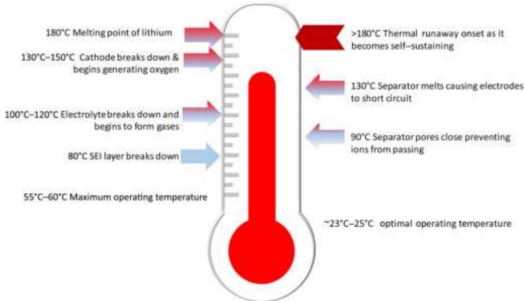
Figure 8. Different stages during thermal runaway [29]
