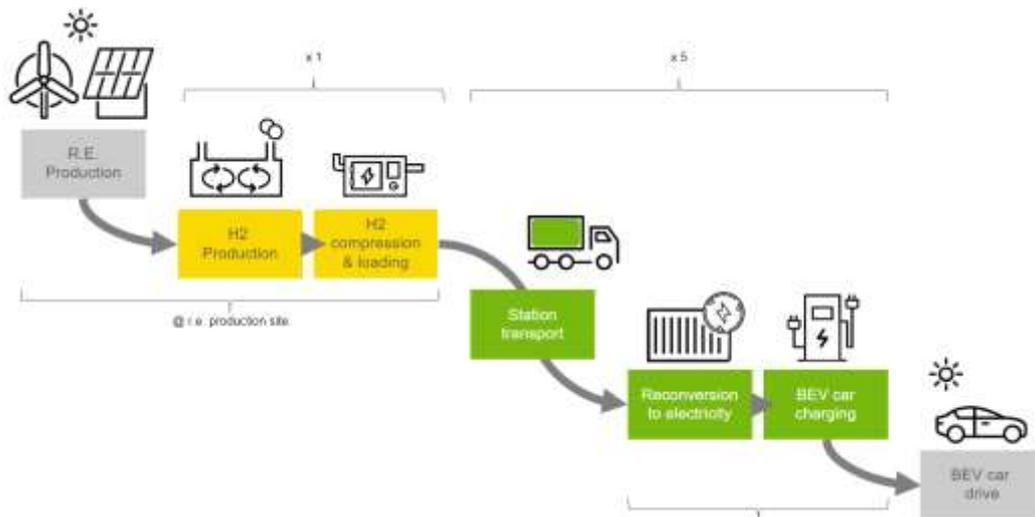
Figure 17. Energy flow process for the hydrogen solution
